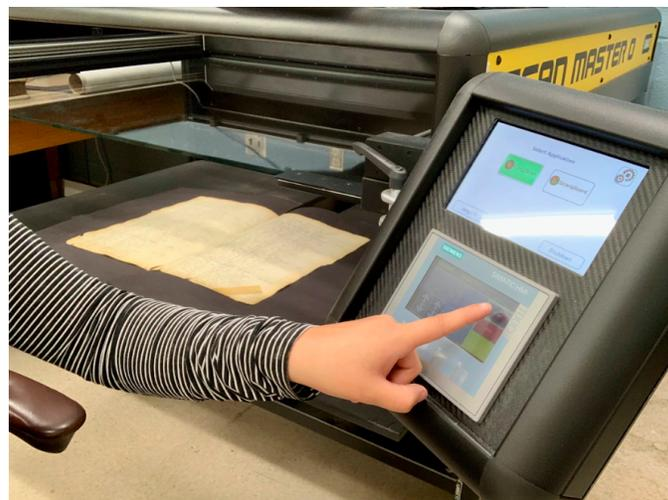
summer. The Scanmaster is a large scanner used for documents and volumes that cannot be put through a normal feed scanner due to their size or fragility. The Kodak scanners were used for smaller items, such as index cards from the card catalog project, that were stable enough to be fed through the machines. I digitized a variety of record types including naturalization records, judicial dockets, marriage licenses, case files, equity papers, artworks, and more.
