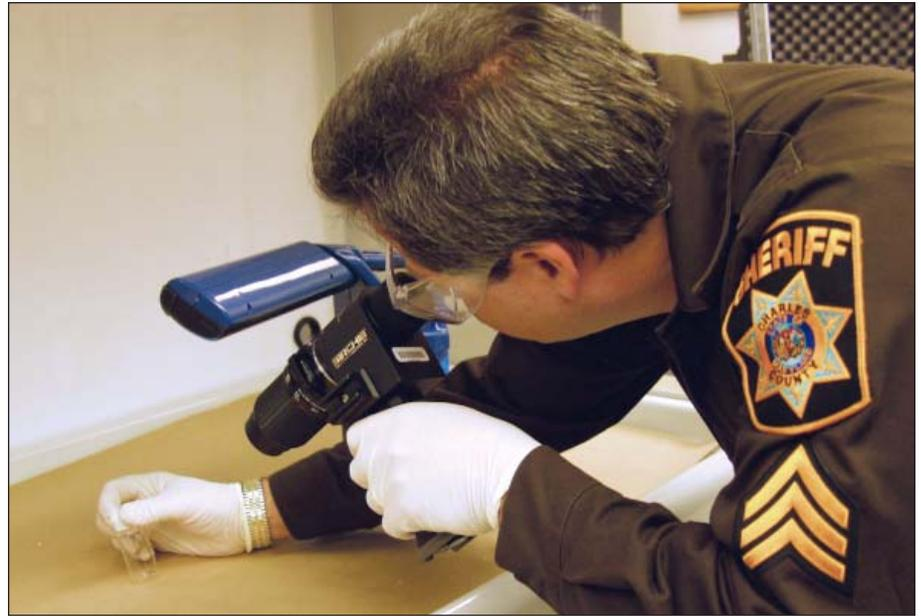
Sgt. Joseph Goldsmith scans evidence for fingerprints with a reflective ultra-violet imaging system. Ultra-violet light travels through filters in the equipment and will illuminate fingerprints in daylight without the need for technicians to pre-process the prints.
