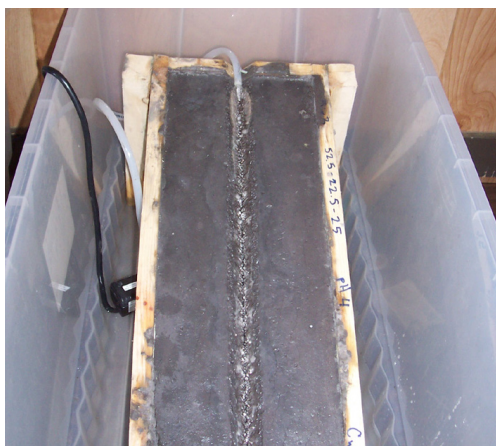
Experimental setup for CCP-grout weathering tests
