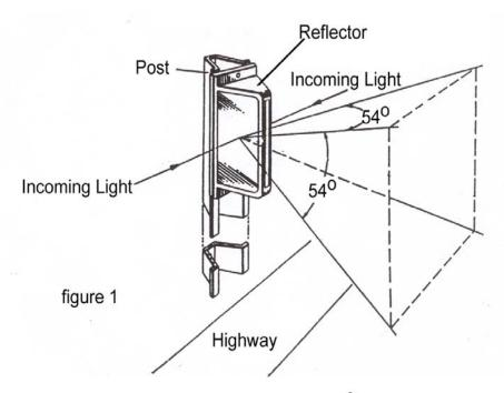
VERTICAL FIELD OF VIEWING shall be 27<sup>0</sup> +/- from the horizontal to the highway. HORIZONTAL FIELD OF VIEWING shall be 27<sup>0</sup> +/- from the perpendicular to the highway.
