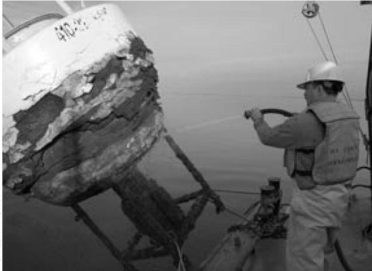
A weather buoy comes aboard after a bad winter in the Chesapeake Bay. Ice fields cut and battered the hull and caused flooding that destroyed the electronics package carried inside.
