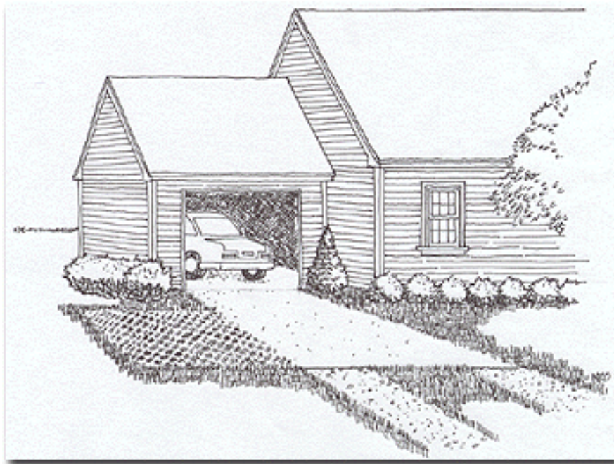
Figure 3: This design for a driveway minimizes impervious surfaces and runoff by using a mix of surfaces including pavers and by keeping a grass median.
