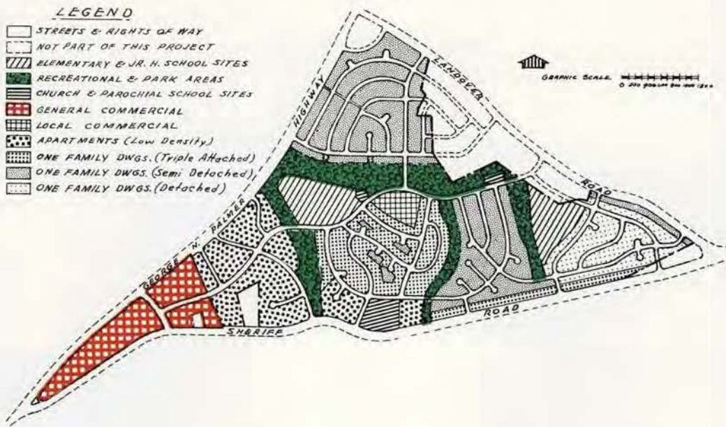
Subdivision plan of the 450-acre Palmer Park development in Prince Georges County. In approving the plan, the Commission, with the cooperation of the developer and his consultants, reserved 53 acres for parks.
