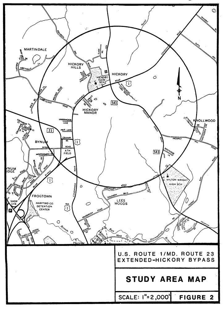
These improvements will be accomplished by relocating US 1 from the Bel Air Bypass to US 1 north of Hickory as a new initial roadway with one 12' lane in each direction to serve ultimately as the two southbound lanes of a four-lane divided highway.
