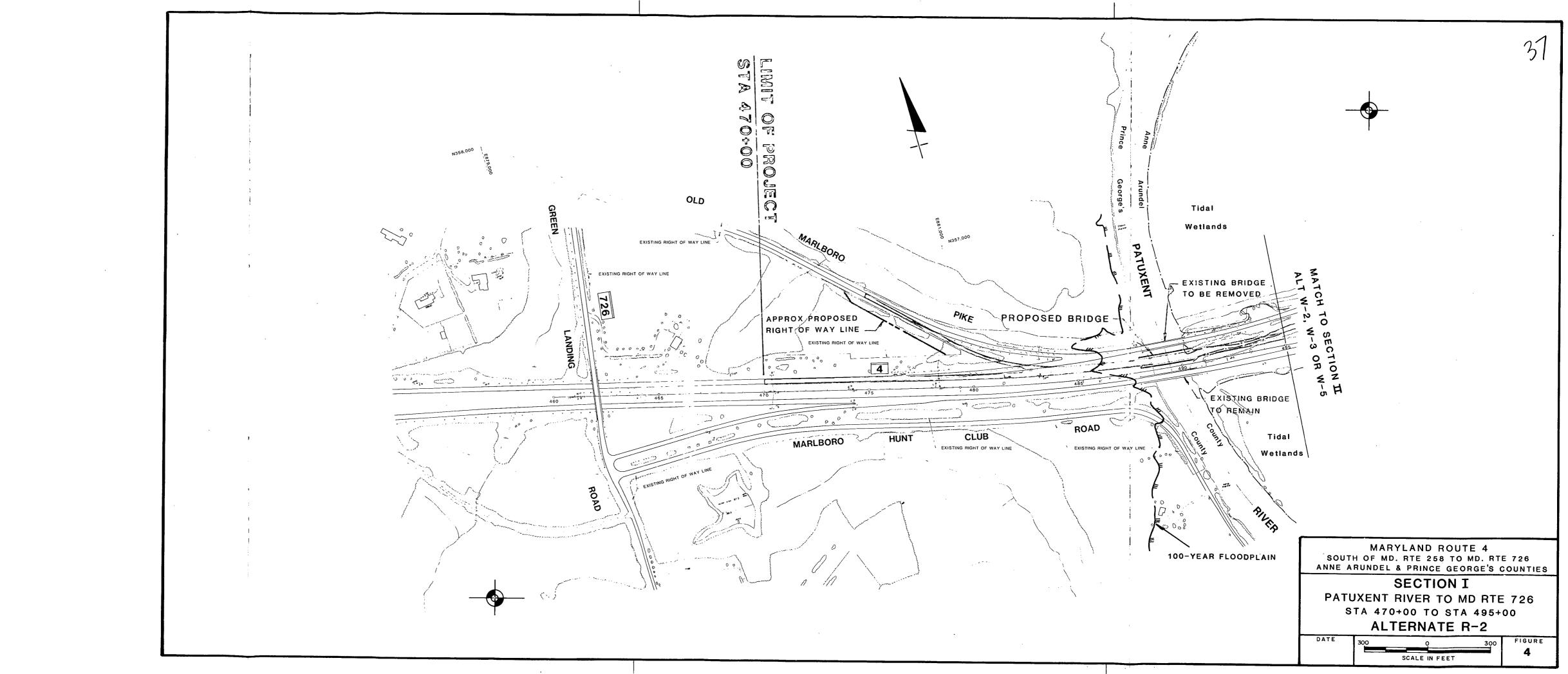
lanes, a deceleration lane, a four foot wide shoulder on the left, and a ten foot wide shoulder on the right. Additionally, this alternate, as presented at the Public Hearing, included widening the existing southbound Maryland Route 4 bridge to provide a full width outside shoulder. The widening will be postponed until such time as deck replacement or complete reconstruction of the southbound bridge is necessary.
