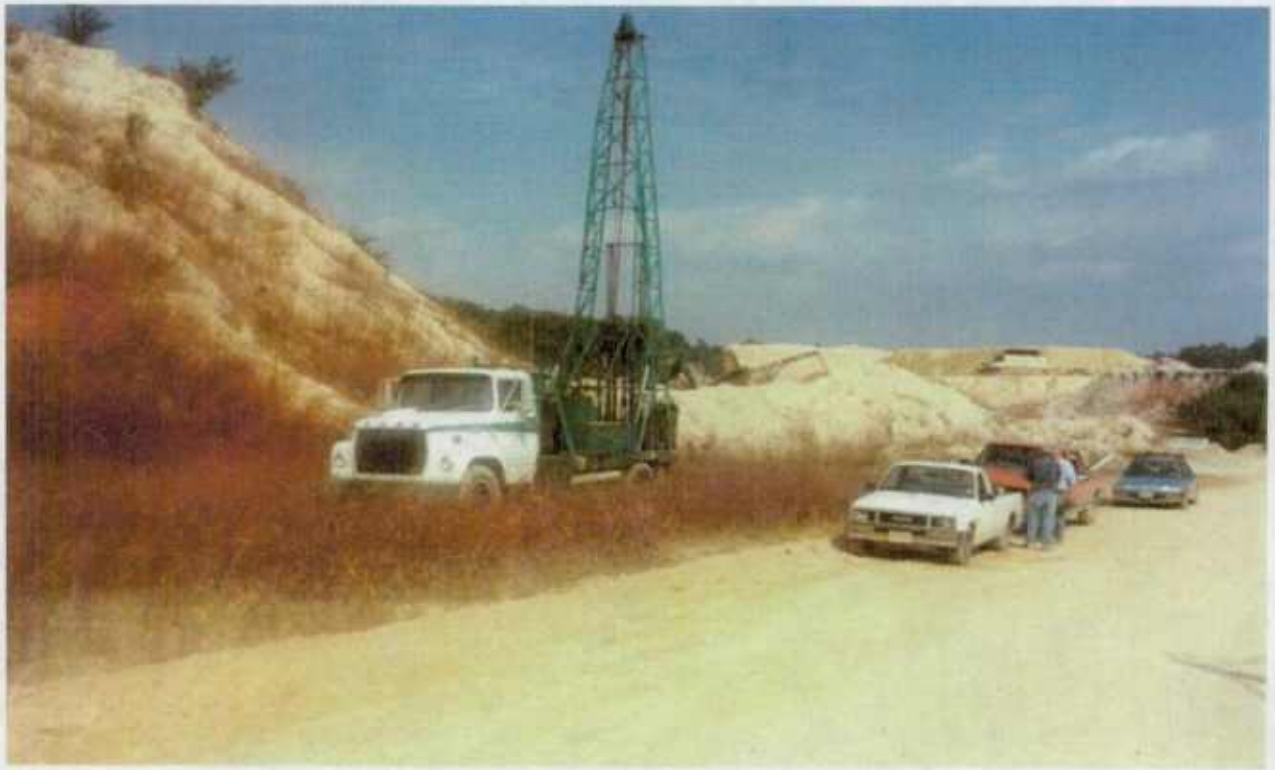
Figure 7.1 – Obtaining Soil Borings at the Furnace Bay Site
