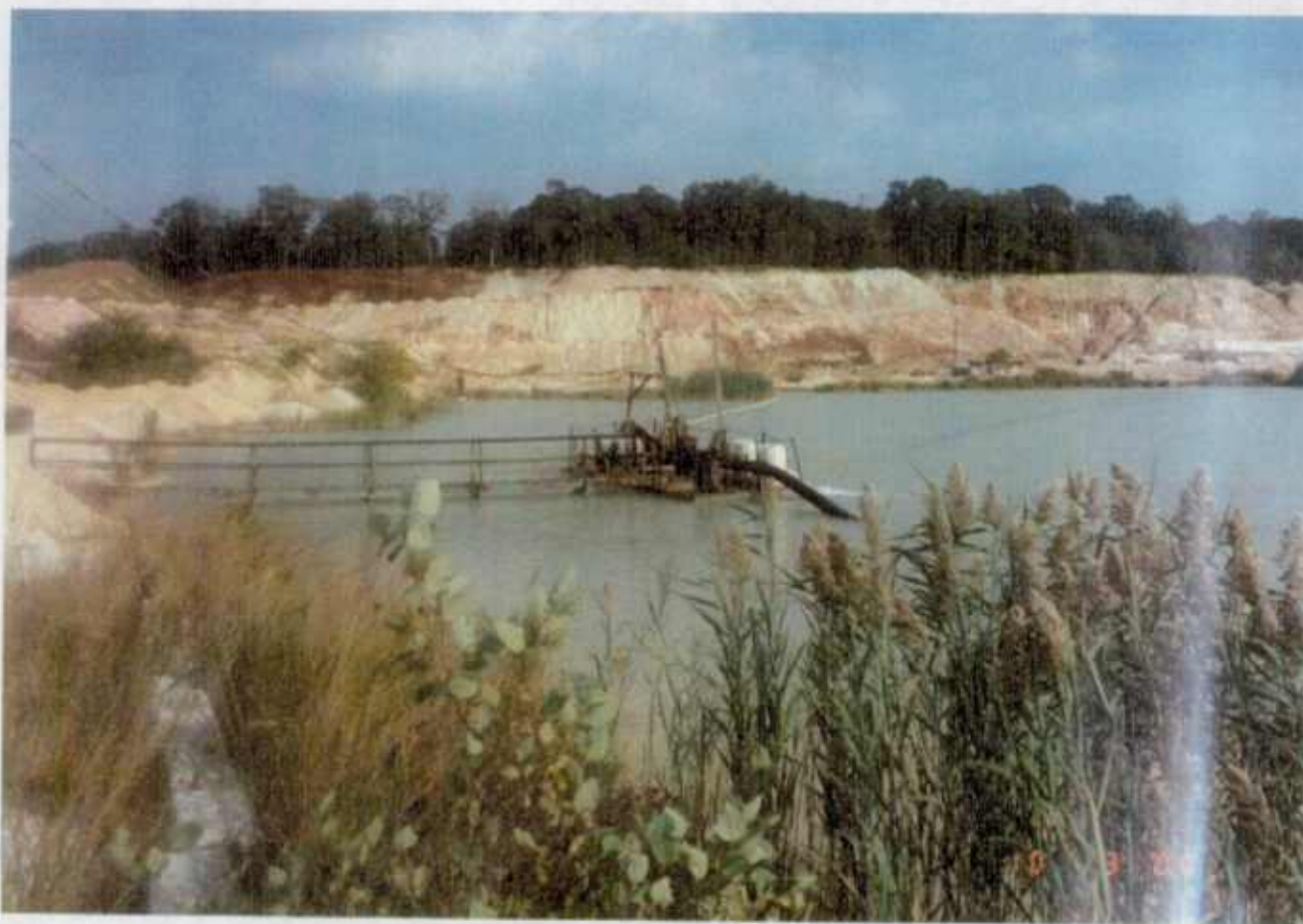
Figure 3.4 – Intake Pumps to Provide Water for Material Processing Operations
