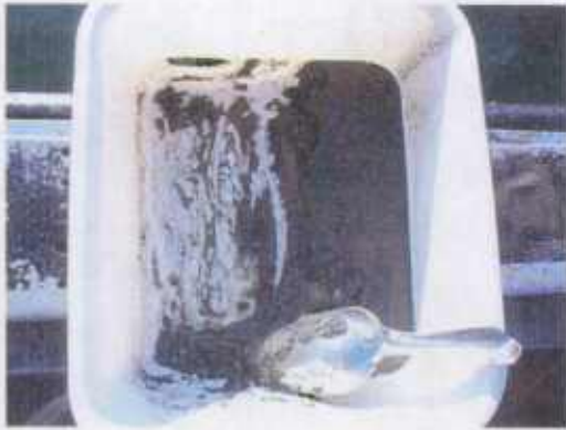
Poplar Island – Sediment at PIM-003 (1500). Sand-silt sediment with clam and shell fragments.
