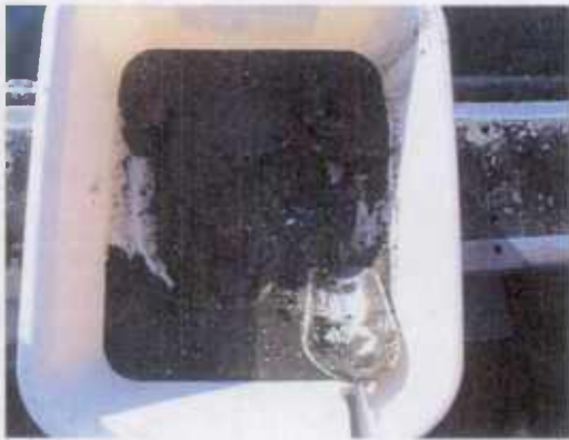
Poplar Island – Sediment at PIM-002 (1420). Sand-silt composition with clam and shell fragments.
