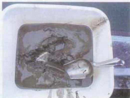
Poplar Island – Sediment at PIM-006 (0845). Mostly silt with some very fine sand particles.
