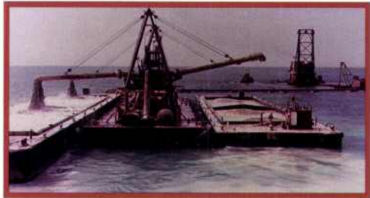
Land Reclamation: The Alaska at work in Kings Bay, Georgia. Using a spider barge (below), the dredge Alaska uses split-hull dump barges for offshore disposal at a project in Colombia. At bottom, a rock cutterhead for 30-inch (760-mm) dredges.
