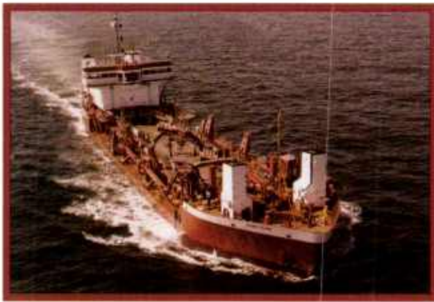
Maintaining and Restoring Material removed from the Sandy Hook Channel by the dredge Sugar Island (below left) was transported to a rehandling area, where it was picked up and pumped to the beach by the Illinois (below right).
