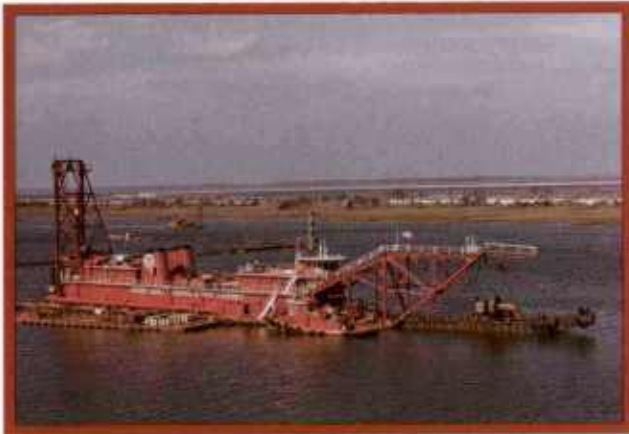
Discharge Diameter 30 in (760 mm) Total Installed Power 11,200 hp (8,300 kW)
