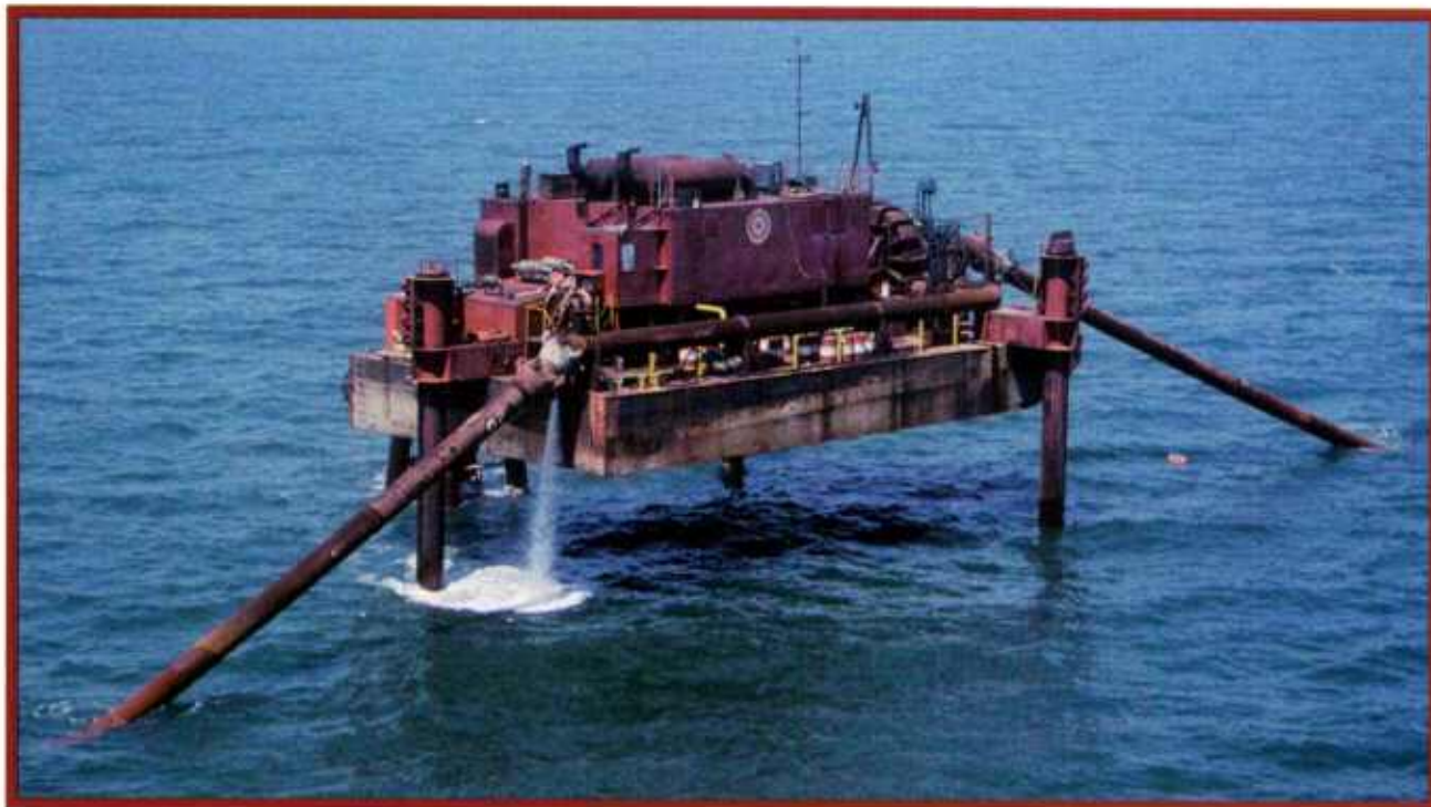
Jack-Up Booster, above, provides more than 4,600 hp (3,400 kW) for pumping material ashore. Her ability to float into position and jack up out of the water enables the booster to be used offshore in exposed waters. Below, Booster No. 2.
