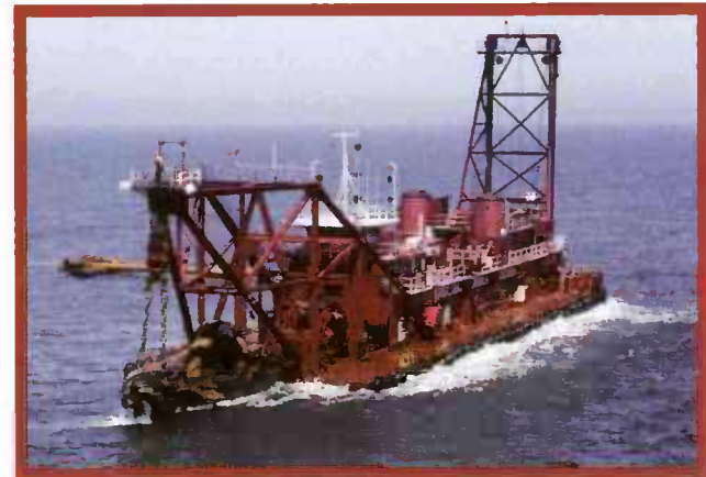
Discharge Diameter 30 in (760 mm) Total Installed Power 11,300 hp (8,400 kW)
