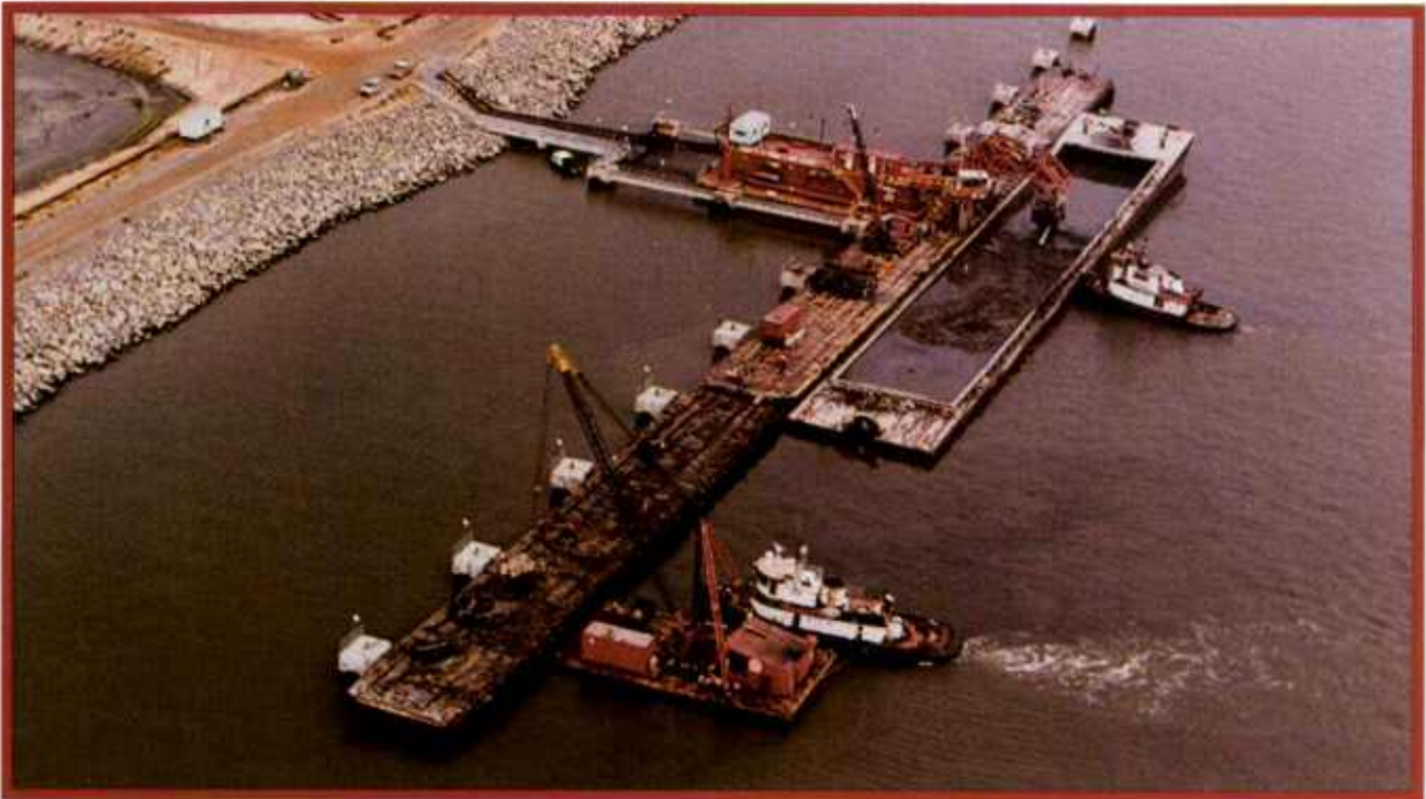
Unloading Capacity: Unloader No. 2 (above) shown where it has done the bulk of the unloading work, at Hart-Miller Island, Chesapeake Bay, Maryland. Below left, a closer view. Below right, Unloader No. 2 setting up for operation in Philadelphia.
