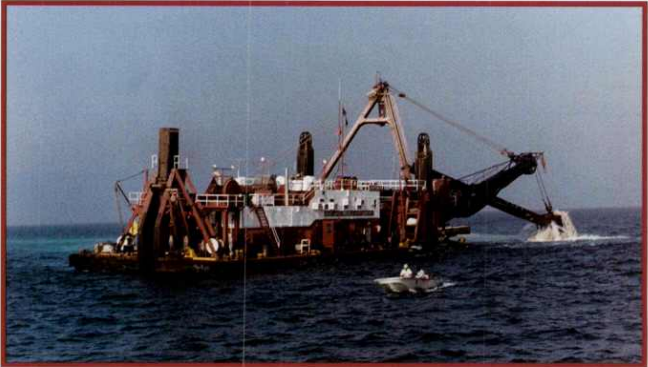
In dipper mode, the dredge Boston digs in the entrance channel to Jebel Ali (above). Below left, the hydraulic cutterhead dredge Georgia; at right, workers on the drillboat Algonquin rig holes drilled in the rock for blasting.
