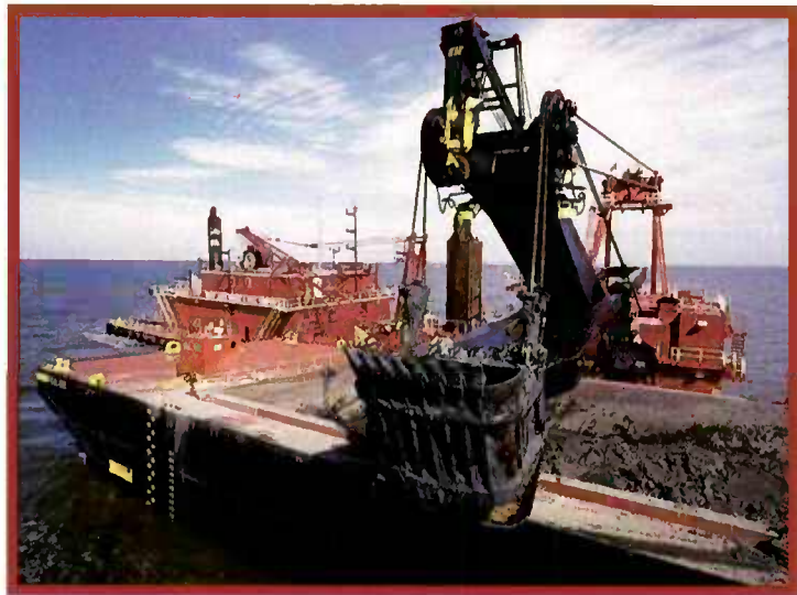
The Chicago can, when necessary, dig directly in unblasted rock with her 18-yd 3 (14-m 3 ) bucket.
