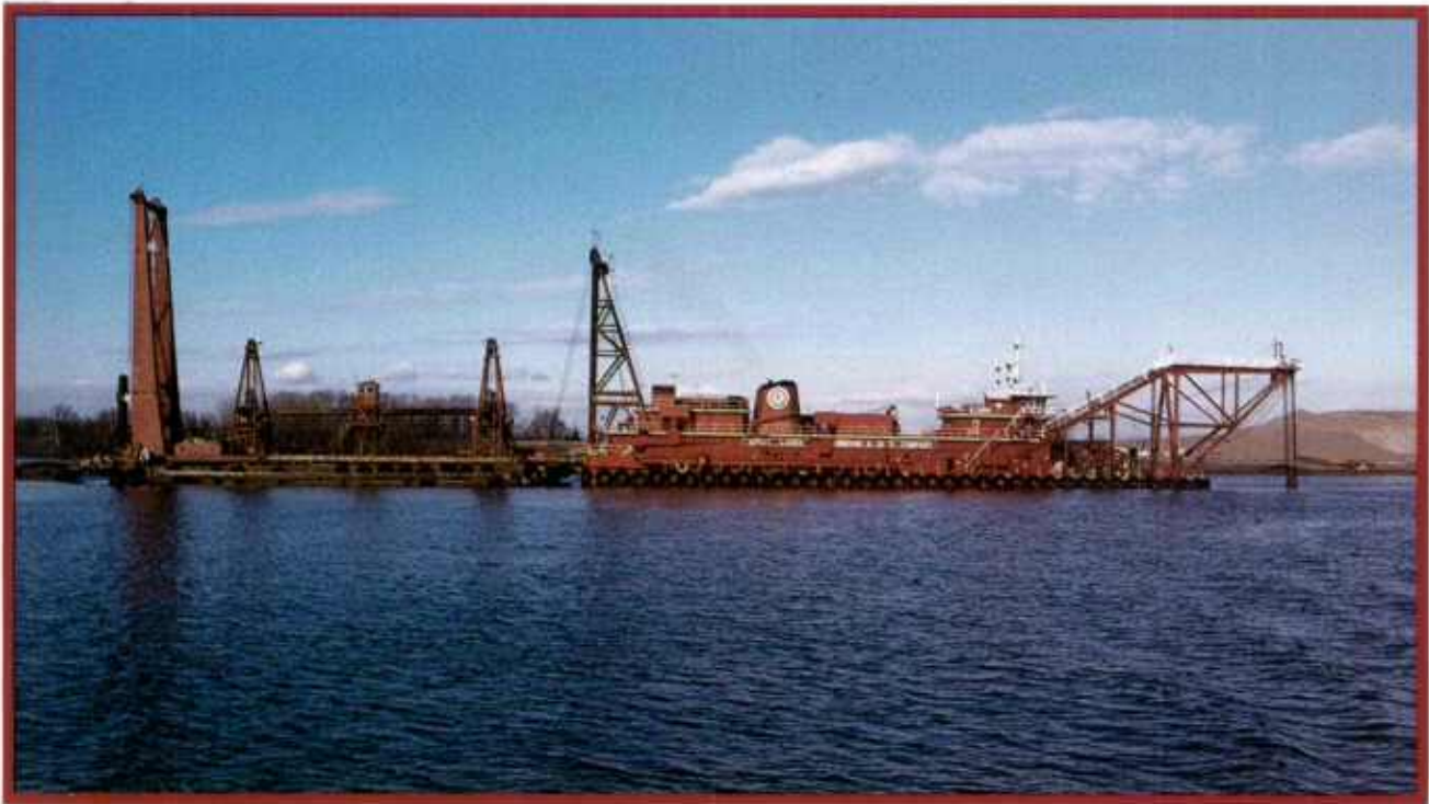
The dredge Illinois is equipped with an extension barge which lengthens the dredge and increases its swing width. The barge also houses towers and piping to enable overboard loading of material barges.
