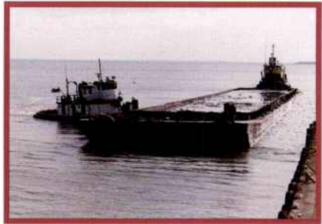
Loading/Unloading: At left, the hydraulic cutterhead Dredge Carolina loads rock into a Series 40 barge. At Hart-Miller Island, a Series 220 material barge is maneuvered into position for hydraulic unloading.
