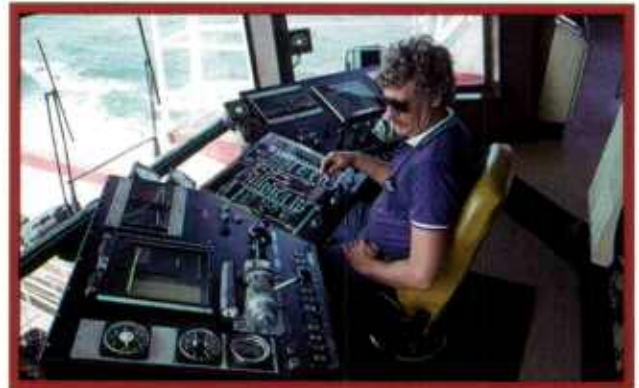
The Dodge Island performs maintenance dredging in the Great Lakes Port of Rochester, N.Y. Her lever room, below, features state-of-the-art electronic control systems. At bottom, one of the dredge's 2,150-hp (1,610-kW) main propulsion engines.
