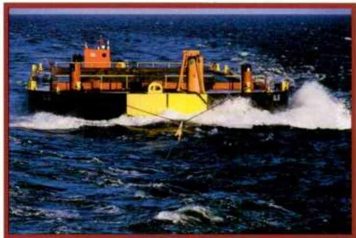
The Chicago's 6,000-yd 3 (4,600-m 3 ) bottom-dump barges are suited for long-haul, high-volume projects. Shown above is a barge fully loaded, en route to a disposal area.
