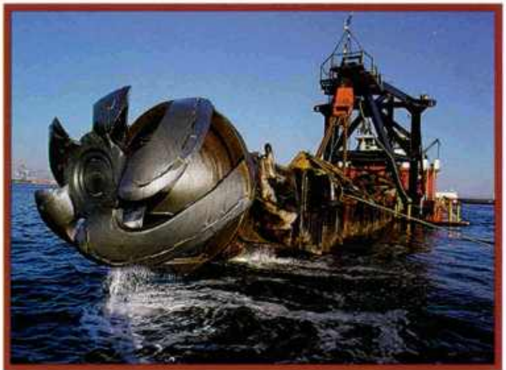
Dredging & Filling: Portions of the fill were along narrow sections of the lining of the facility. Below, left, Dredge No. 53 removed unsuitable material from under the rock perimeter wall. At right, a clay material cutterhead of the dredge Florida.
