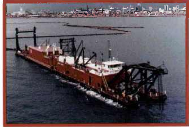
Discharge Diameter 36 in (910 mm) Total Component Power Installed 16,115 hp (12,022 kW)
