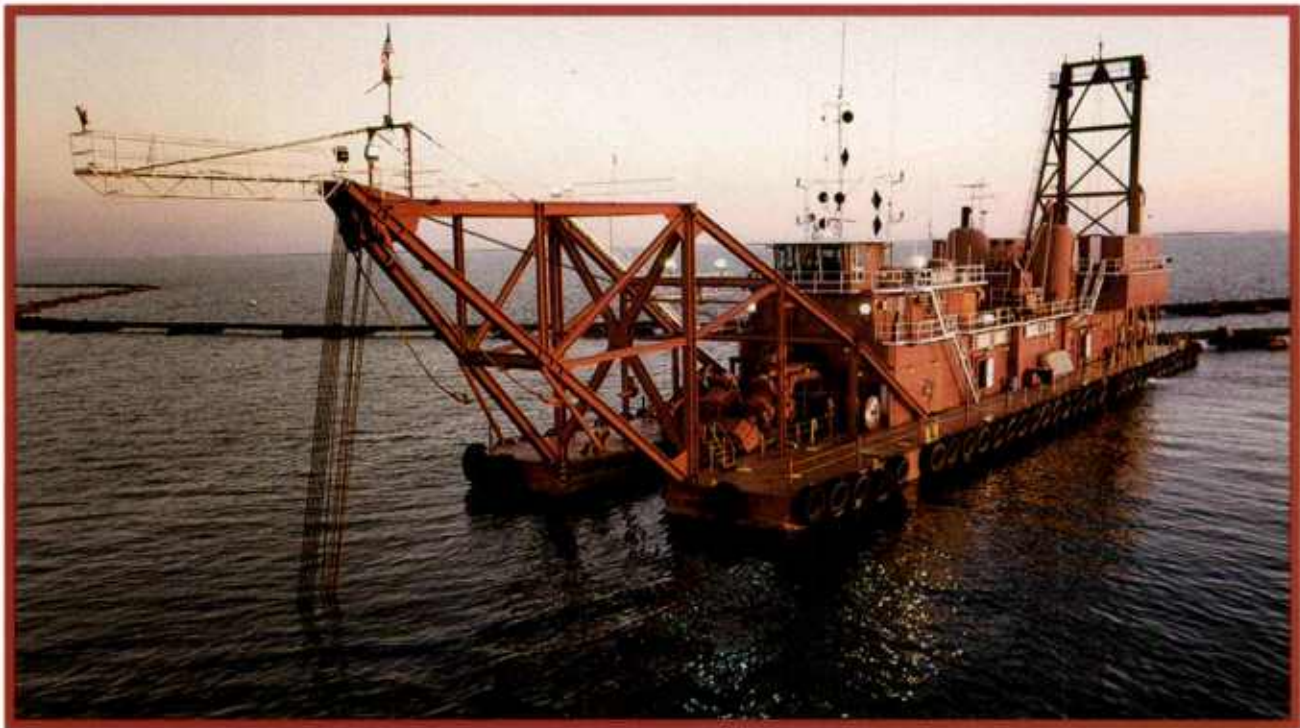
The Dredge Alaska is particularly well suited for offshore work in rough conditions, and can pump material up to 30,000 ft (9,100 m).
