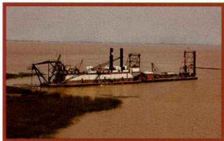
Hydraulic cutterhead dredge New York removing nearshore material at Buenos Aires.
