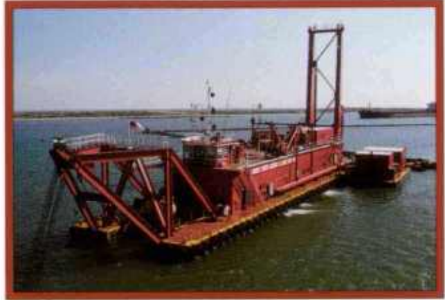
Discharge Diameter 30 in (760 mm) Total Component Power Installed 14,652 hp (10,930 kW)
