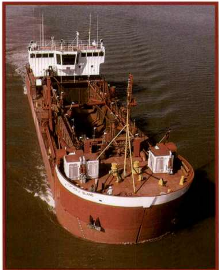
The Northerly Island features integral pump-out as well as split-hull bottom-dump material disposal.
