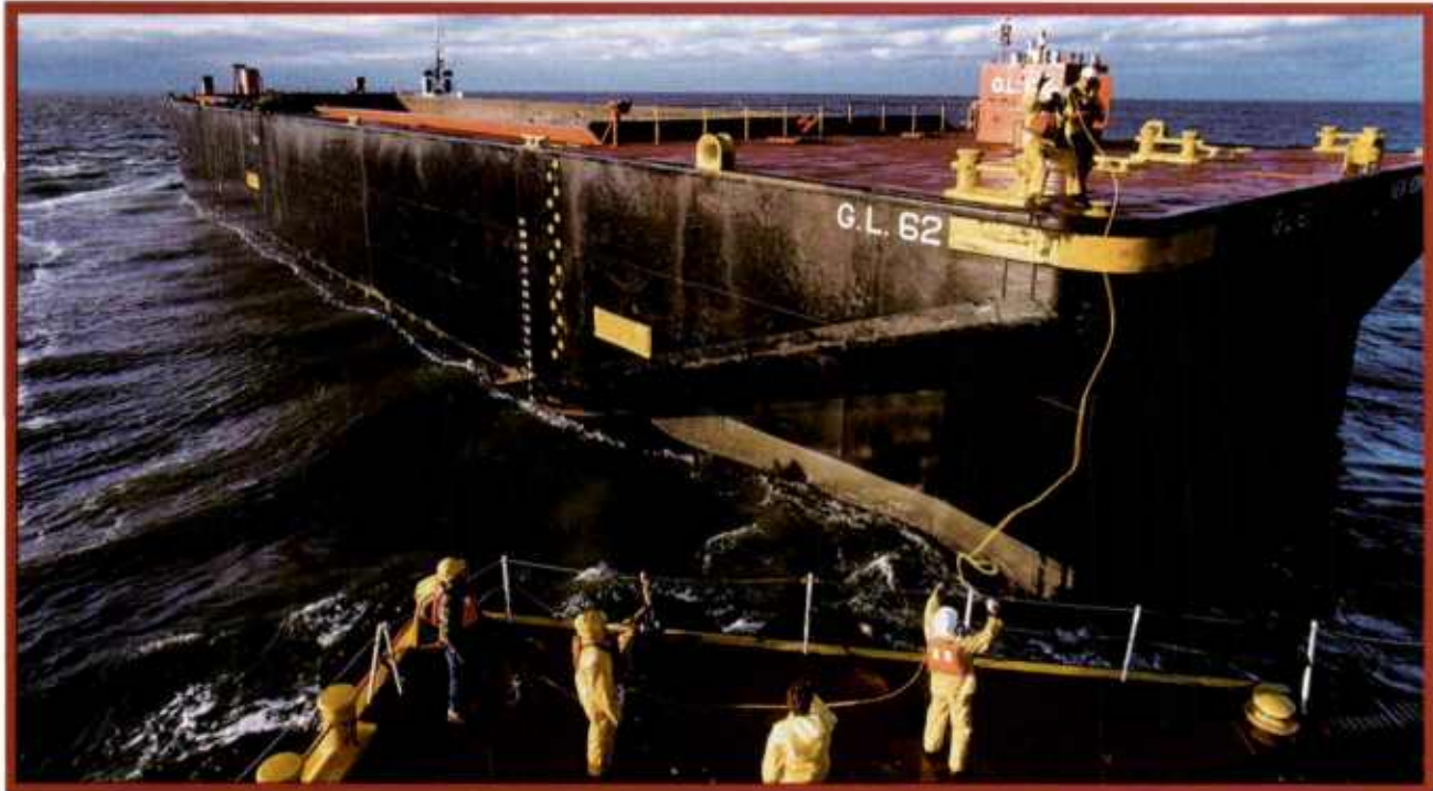
A Vast Barge Fleet: Great Lakes owns a total of 43 material transport barges, ranging in size from the 6,000-yd 3 (4,840-m 3 ) unit above to 1,540-yd 3 (1,175 m 3 ) units. Their configurations include split-hull, bottom-dump, 6-, 7- and 8-pocket bottom door dumpers and miscellaneous hopper units.
