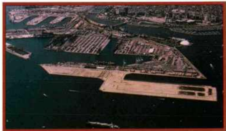
Pier J in Progress: The dredge Florida (visible at top center) pumps sand into the main fill. Below, after completion of the project, the 120-acre (50-hectare) plot undergoes development. At bottom, the Florida at work early in the project.
