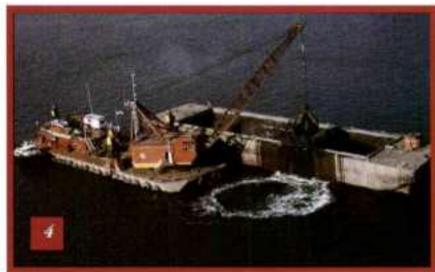
A Versatile Barge Fleet: 1) One of Great Lakes' Series 90 2,000-yd 3 (1,530-m 3 ) rock barges loaded in New York Harbor. 2) A Series 60 6,000-yd 3 (4,840-m 3 ) barge splits its hull to dump material. 3) Series 60 barge working with the Dredge Chicago. 4) Series 30 4,000-yd 3 (3,060-m 3 ) barge with Dredge No. 54.
