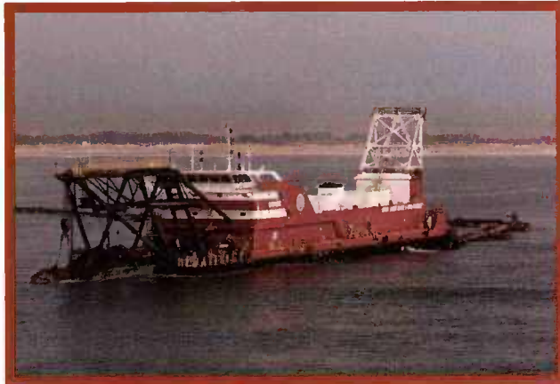
Discharge Diameter 30 in (760 mm) Total Installed Power 15,325 hp (11,432 kW)
