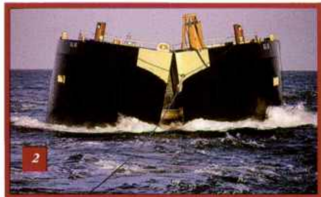
A Vast Barge Fleet: Great Lakes owns a total of 43 material transport barges, ranging in size from the 6,000-yd 3 (4,840-m 3 ) unit above to 1,540-yd 3 (1,175 m 3 ) units. Their configurations include split-hull, bottom-dump, 6-, 7- and 8-pocket bottom door dumpers and miscellaneous hopper units.
