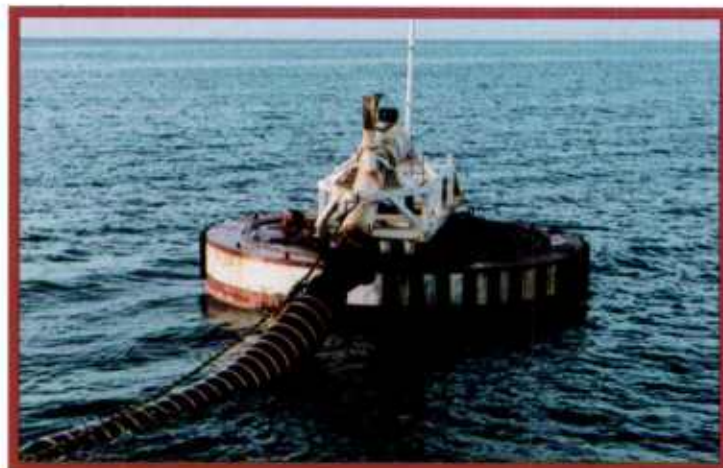
Pump-Out: The Long Island discharges sand for the beach at Ocean City through a Self-Contained Offshore Transport System (SCOTS) Buoy (below), which is connected to a submerged pipeline running to the beach. At bottom, a discharge site at Ocean City.
