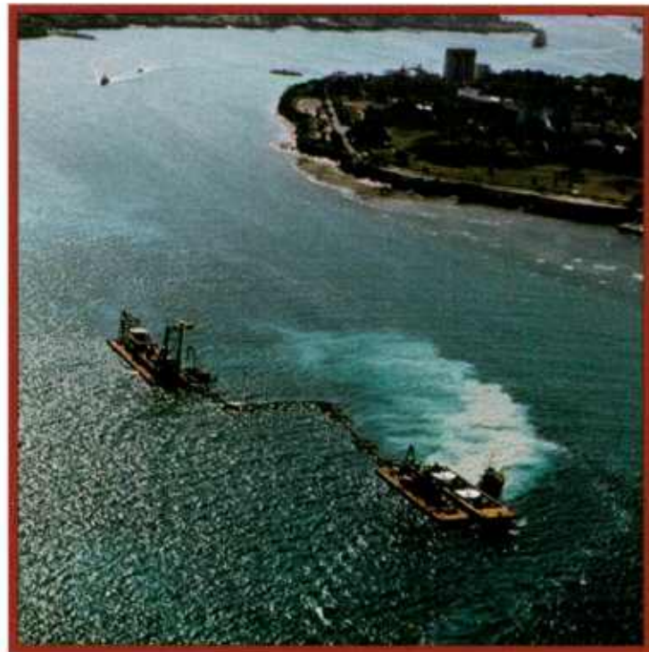
The Alaska feeds material to barges by means on a spider barge.
