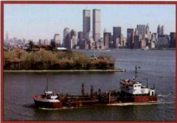
The trailing suction hopper dredge Northerly Island (above) transports material for placement. At right above, the hydraulic cutterhead dredge Georgia excavated silts and sand on the project. Below right, clamshell Dredge No. 50 removes material preparatory to placement of fill and armor stone.
