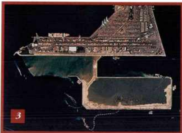
Pier J Takes Shape: This sequence shows the development of Pier J over a 9-month period. (1) The rock perimeter wall begins to emerge. (2) The future outline of the facility becomes visible. (3) Fill along the outer edges of the southern portion breaks the surface. (4) The project nears completion. A container facility is to be built on the site, which is part of the port's long-term 2020 Expansion Program.
