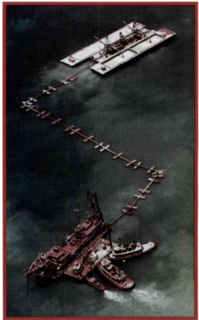
Long-haul disposal via barges can be accomplished through the use of a spider barge loading system, shown here at work with the Georgia in Dubai, U.A.E.. Below, the Georgia in tight quarters.
