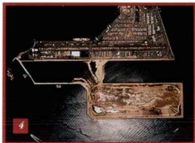
Pier J Takes Shape: This sequence shows the development of Pier J over a 9-month period. (1) The rock perimeter wall begins to emerge. (2) The future outline of the facility becomes visible. (3) Fill along the outer edges of the southern portion breaks the surface. (4) The project nears completion. A container facility is to be built on the site, which is part of the port's long-term 2020 Expansion Program.
