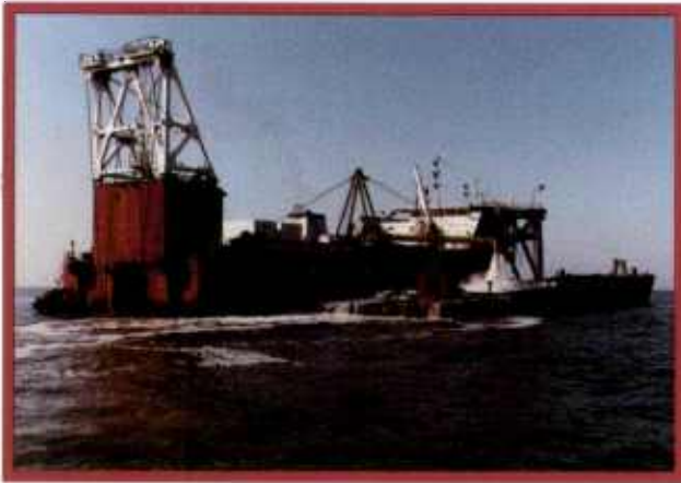
Loading/Unloading: At left, the hydraulic cutterhead Dredge Carolina loads rock into a Series 40 barge. At Hart-Miller Island, a Series 220 material barge is maneuvered into position for hydraulic unloading.
