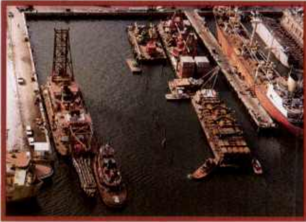
Positioning equipment for loading onto semi-submersible vessel.
