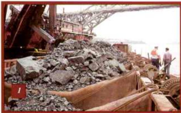
A Vast Barge Fleet: Great Lakes owns a total of 43 material transport barges, ranging in size from the 6,000-yd 3 (4,840-m 3 ) unit above to 1,540-yd 3 (1,175 m 3 ) units. Their configurations include split-hull, bottom-dump, 6-, 7- and 8-pocket bottom door dumpers and miscellaneous hopper units.
