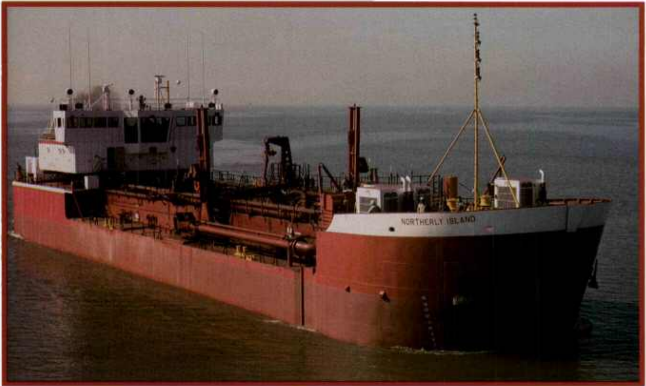
The Northerly Island features integral pump-out as well as split-hull bottom-dump material disposal.
