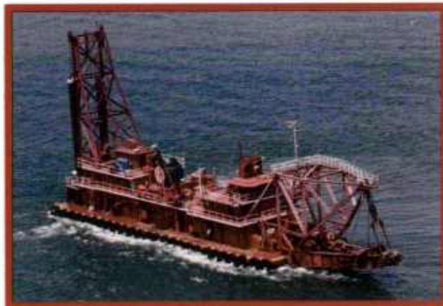
Discharge Diameter 26 in (660 mm) Total Installed Power 6,800 hp (5,060 kW)
