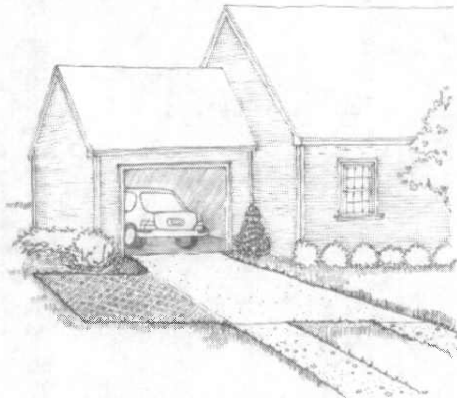
Figure 3: This design for a driveway minimizes impervious surfaces and runoff by using a mix of surfaces including pavers and by keeping a grass median.
