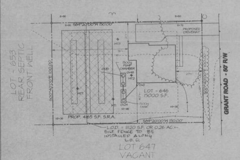
\*\*\*\*\* MOUND MUST BE CONSTRUCTED \*\*\*\*\* PRIOR TO DRILLED WELL INSTALLATION
