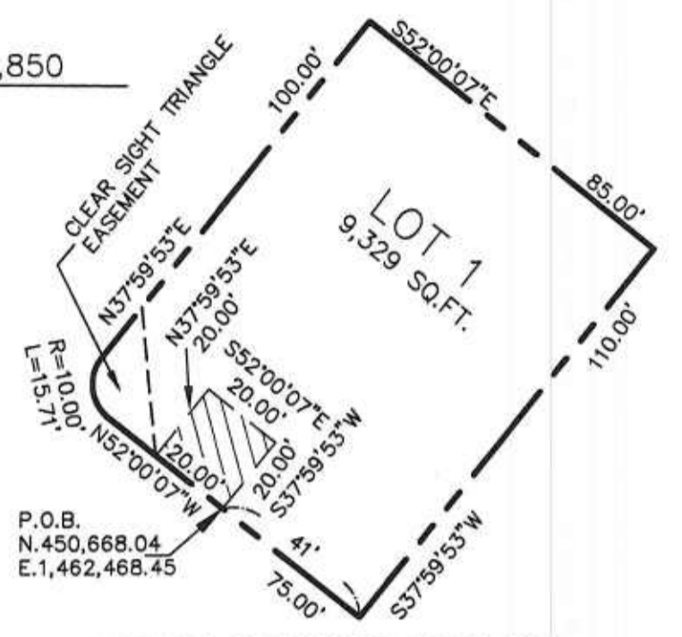
UTILITY EASEMENT LOCATION SCALE: 1"=40'
