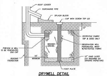
NTS FANDARD DIMENSIONS FDR 1,000 SQ. FT. ROOFTOP AREA (MAXIMUM ALLDWED ) " W x 10' L x 4' D DR 200 C. F. (WITH A VOID RATIO DF D.4D) PROVIDES 8D F. DF STORACE VOLUME PER DRYWELL
