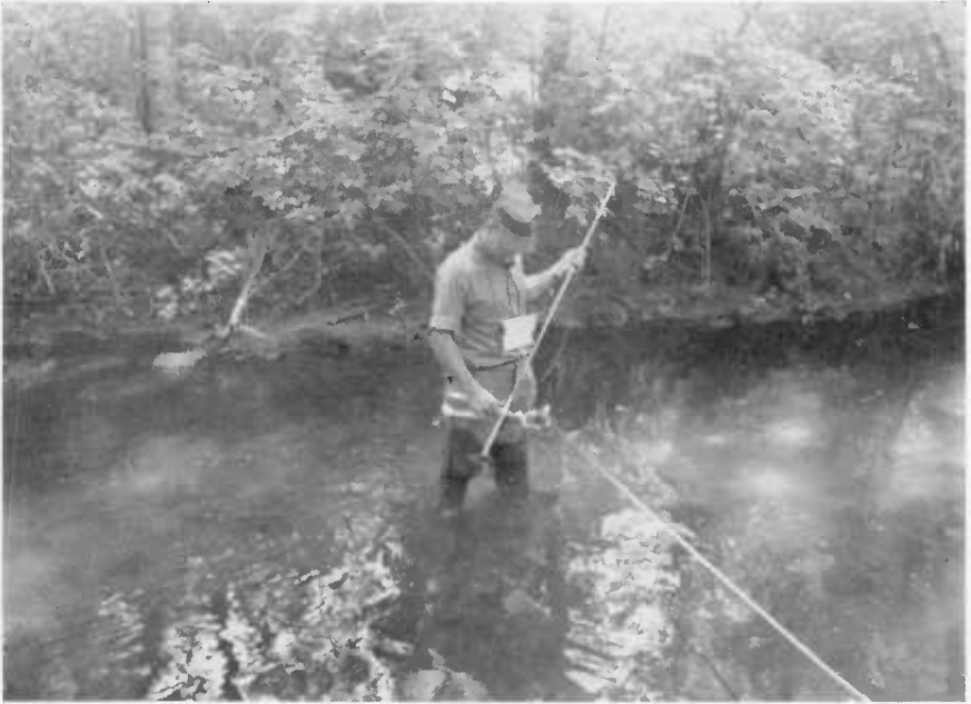
FIGURE 1. Engineer Making Discharge Measurements by Wading
