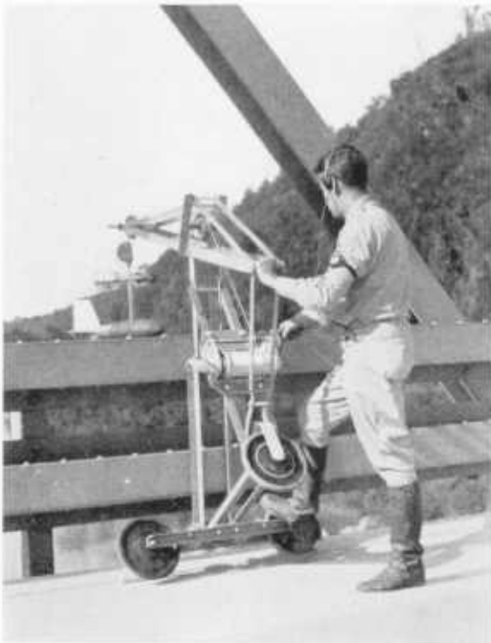
FIGURE 2. Highway Bridge Equipment Used to Measure Discharge at Stages Higher than Wading
