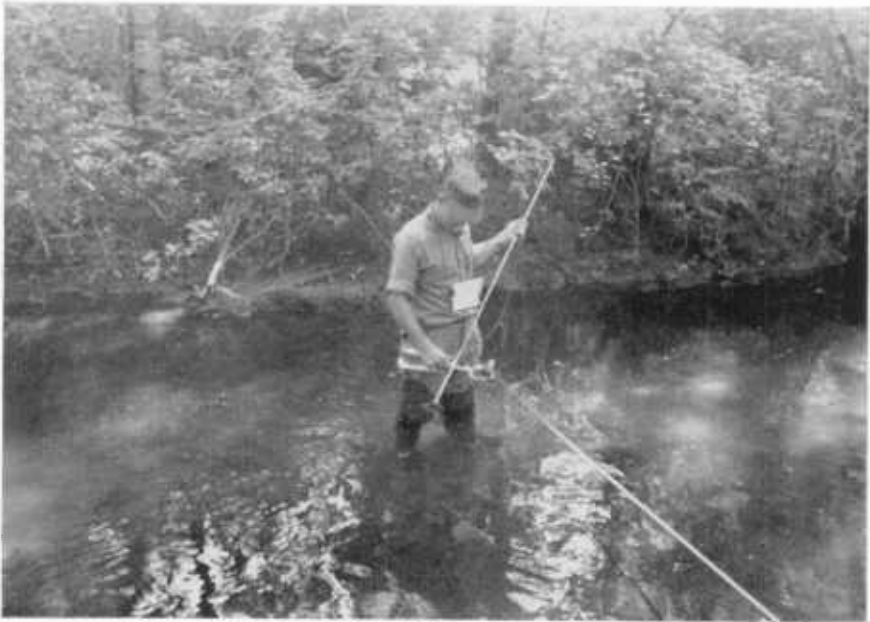
FIGURE 2. Engineer making Discharge Measurements by Wading
