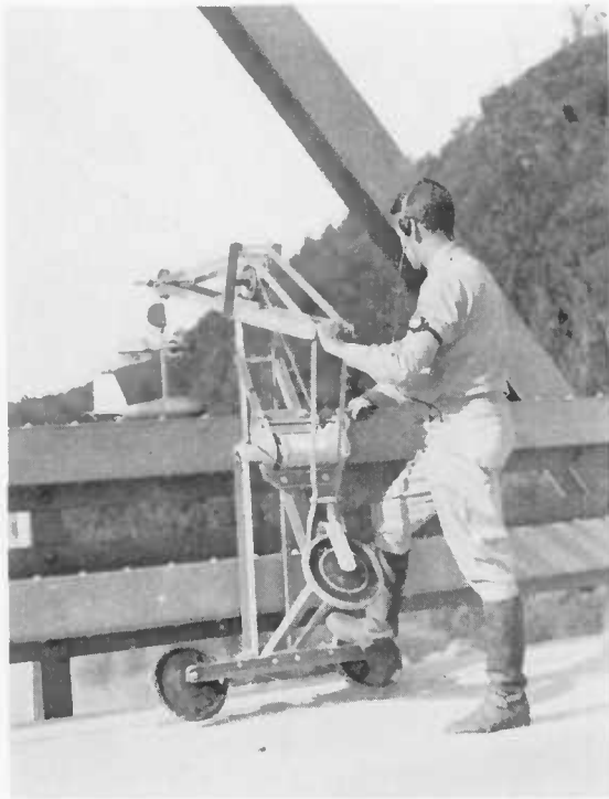
Fig. 2. Highway Bridge Equipment Used to Measure Discharge at Stages Higher than Wading
