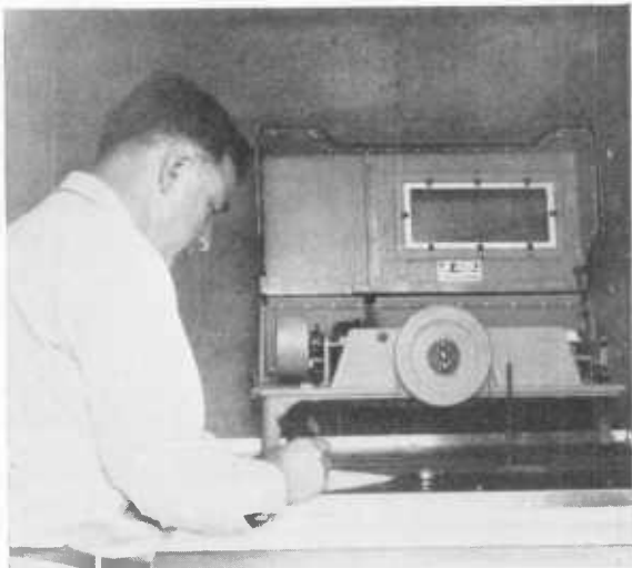
FIGURE 2. Engineer inspecting automatic water-stage recorder.
