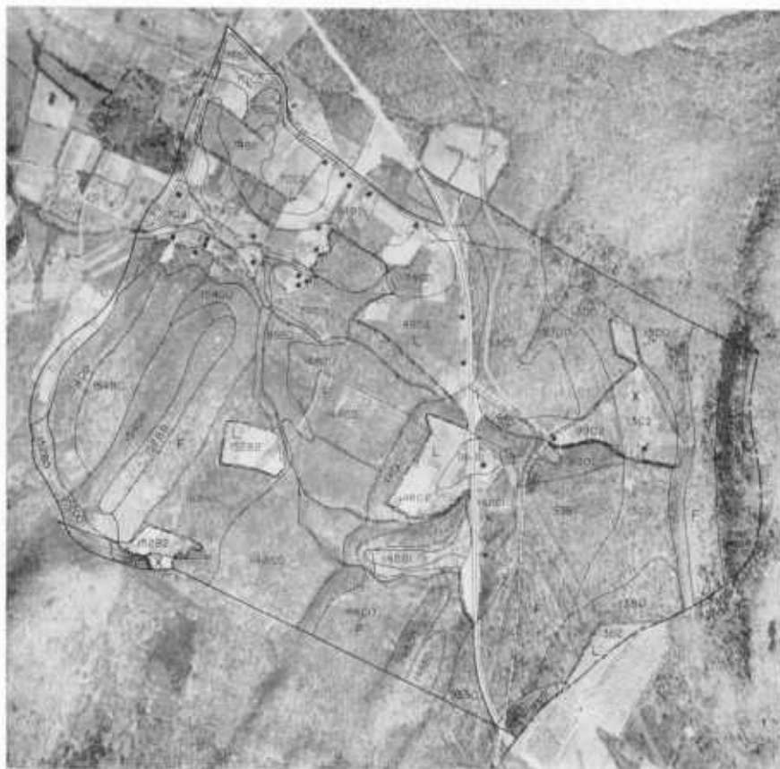
PLATE 23. Farm Planning Conservation Survey Map in the South Mountain Area. Shows pattern of slopes and associated soil, erosion and land use conditions. Soil, slope, and erosion boundaries are shown by solid lines and land use by dashed lines. First number in compound symbol is soil type. Deep, well-drained, acid soils: 28, Highfield gravelly loam; 74, Allen gravelly loam. Moderately deep to shallow, imperfectly drained soil, having hardpan in subsoil: 70, Trego gravelly silt loam.
