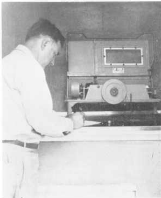
Figure 2. Engineer Making Inspection of Automatic Water-Stage Recorder
