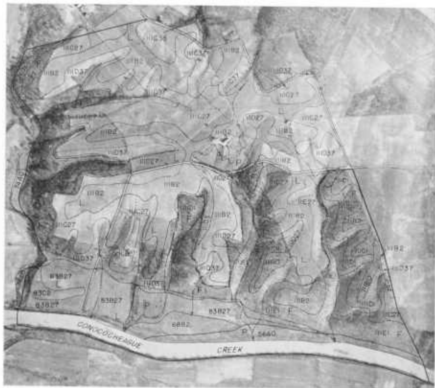
PLATE 27. Farm Planning Conservation Survey Map in the Martinsburg Shale Area of the Great Valley. Shows pattern of slopes and associated soil, erosion, and land use conditions. Soil, slope, and erosion boundaries are shown by solid black lines and land use boundaries by dashed lines. First number in compound symbol is soil type.
