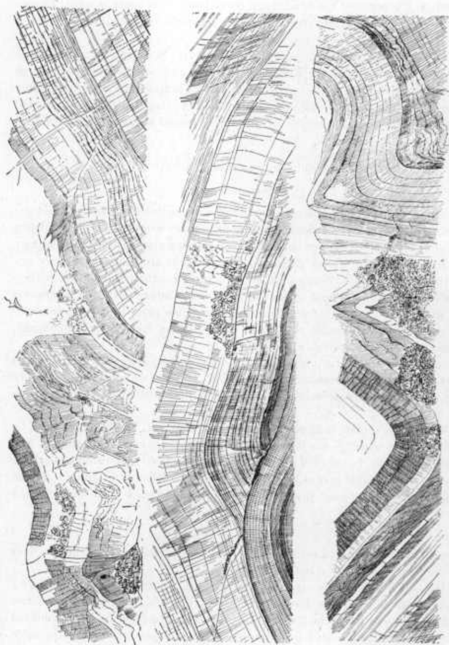
FIGURE 28. Drawing of Central Portion of Cacapon Section. Will's Creek shale. Competent beds in flexure folds, incompetent beds in shear folds with axial plane cleavage. Thrusts follow bedding planes and eliminate some portions of the section. Thrusts seem to be early because some of them are intensely folded.
