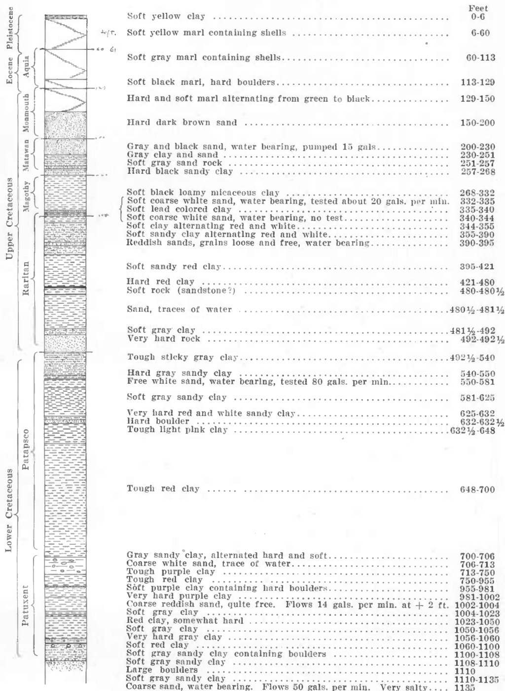
Fig. 1.—Section of the Deep Well at Chestertown.
