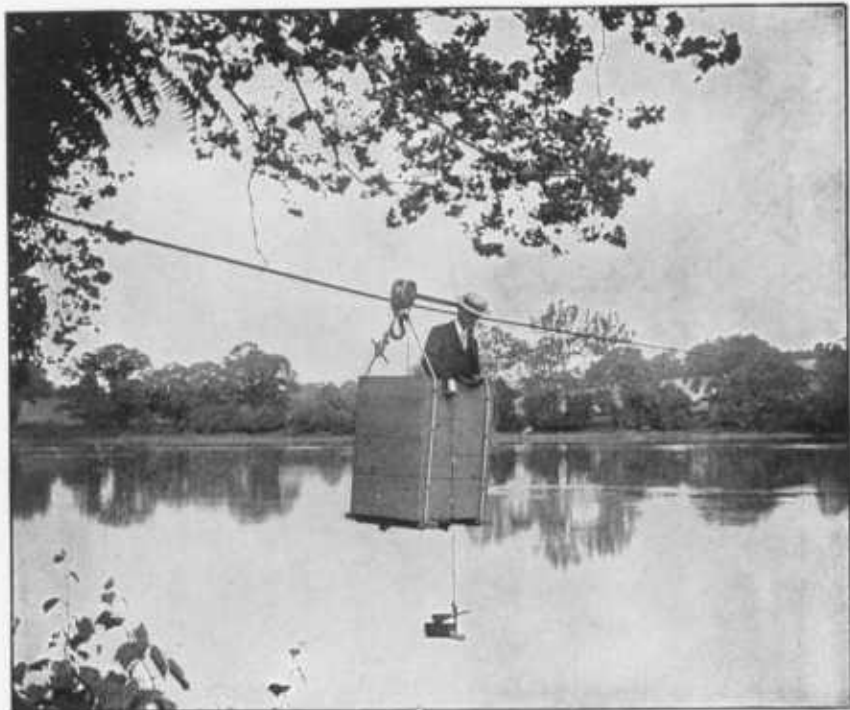
FIG. 1.—CAR USED IN MEASURING VELOCITY OF RIVER WATER.
