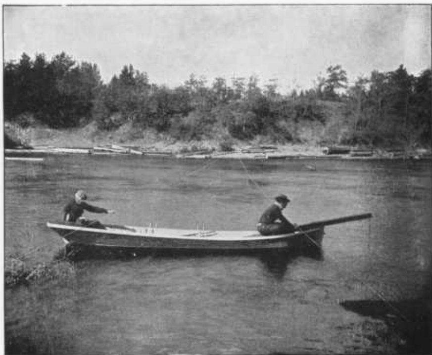
FIG. 2.—MEASURING VELOCITY OF RIVER WATER FROM BOAT.
