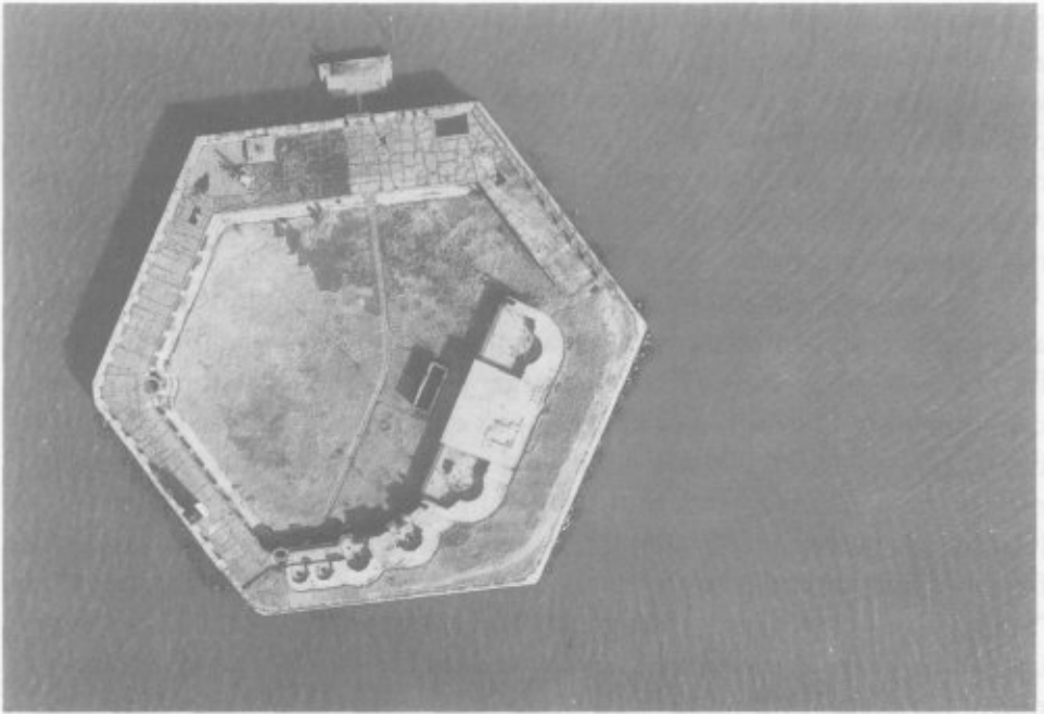
Aerial view of Fort Carroll taken in 1937. Behind the emplacements for a battery of twelve-inch guns is a power house. A lighthouse tower is visible on the southwest face, and the dock off the north face. (Enoch Pratt Free Library.)
