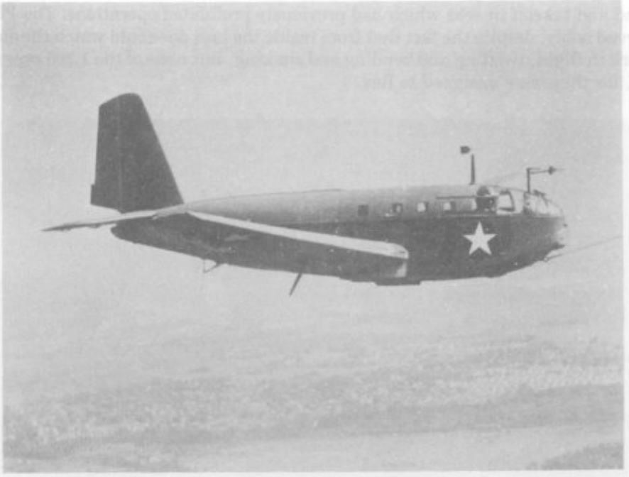
Allied Aviation Corporation's XLRA, a plywood glider. U. S. Navy.
