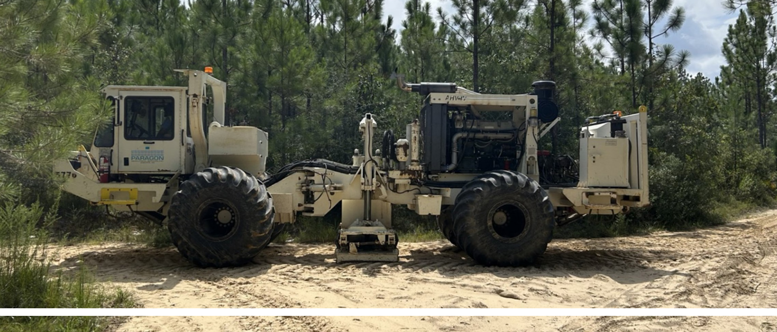
A vibroseis truck utilizes low-frequency vibrations to acquire data at the project location in northern Mobile County, Alabama.
