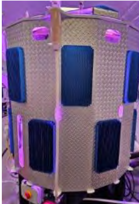
One of several algae growing tanks at Ferry Cove Oyster Hatchery. This algae feeds the oysters through many stages of life.
