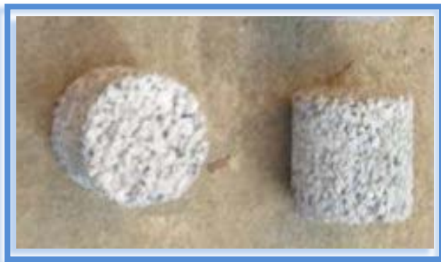
Figure 5-17 Pervious Concrete Test Cylinders Made with CCBs
