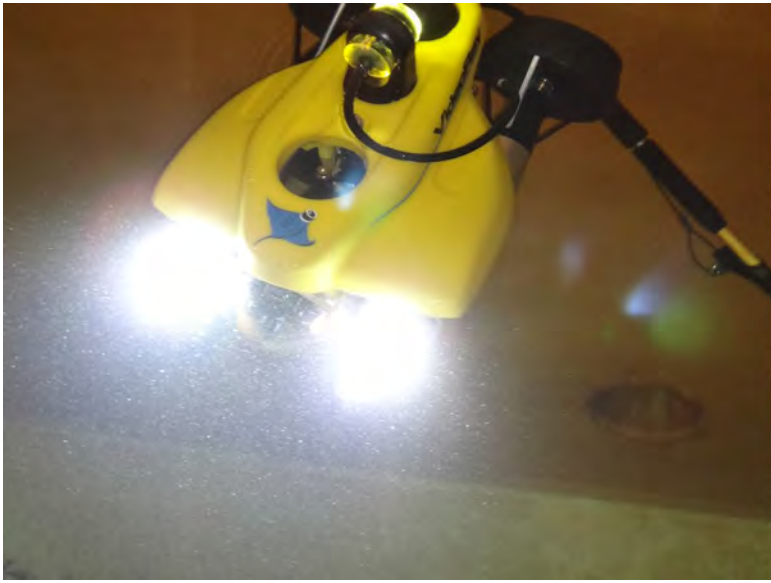
VideoRay equipment allows remote water tank inspections
