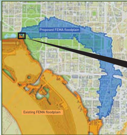
Image of FEMA floodplain area in the monumental core reflecting the existing area and the proposed floodplain if upgrades aren't made to the system of temporary closures.
