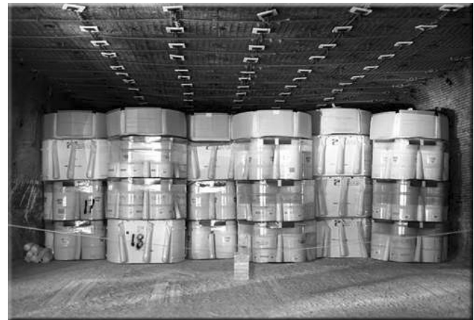
Drums of transuranic waste are stacked in a disposal room where salt will eventually flow and permanently encapsulate the containers. Photo courtesy of the U.S. Department of Energy.
