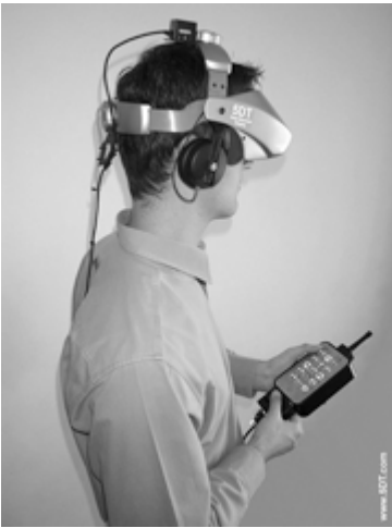
Virtual Reality Training Simulators are the next generation of miner training equipment. The trainee views the virtual Long Wall and its surroundings with a Head Mounted Display. The trainee controls the virtual Long Wall with a real Shearer Remote Control that is interfaced with the host simulation computer. Images courtesy of Fifth Dimension Technologies, www.5DT.com .
