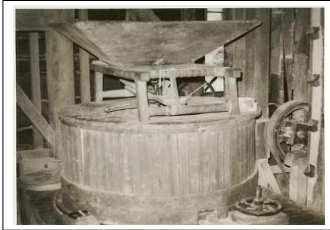
Millstone vat and hopper, Wye Mill.
