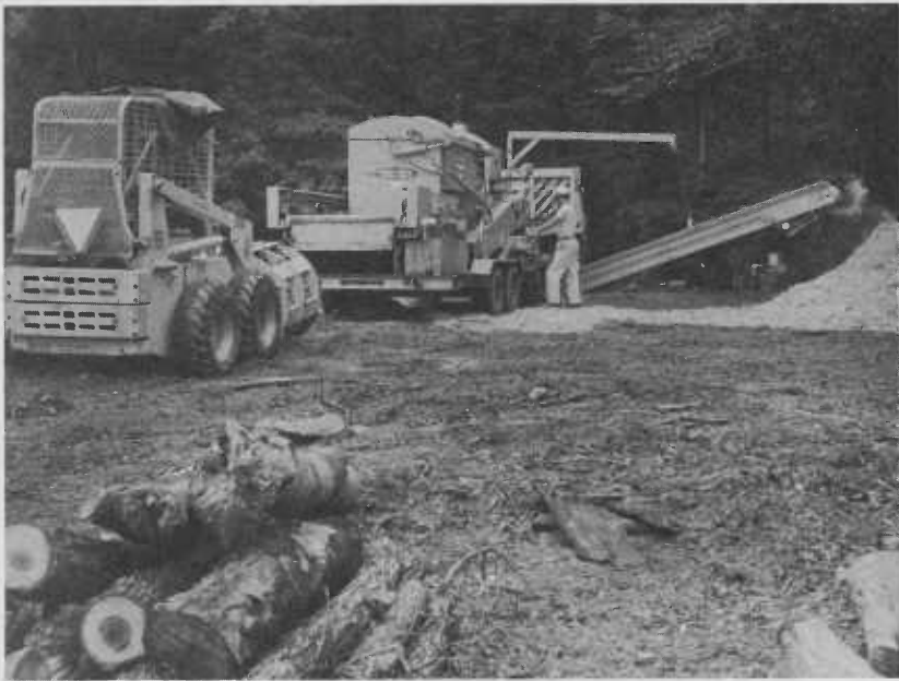
The Vermeer Log Grinder shown in operation aids in the complete ecological recycling of dead trees.
